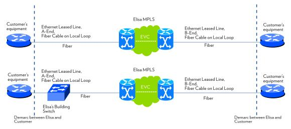
The handover interface is confirmed in the delivery confirmation/notification of completion. The nominal speed of the service is the same at both A-and and B-end.
