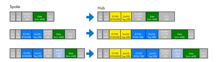
At hub subscription, each frame format has one additional VLAN field, as seen in picture above. This VLAN identifier (or q-tag) is used for identifying the related spoke subscription. This arrangement is illustrated in the diagram below.
