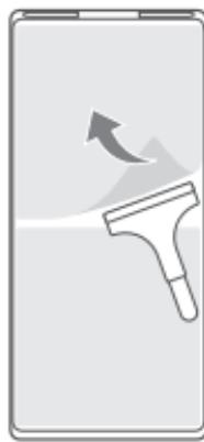
5. Spray adhesive removal to the glass and the adhesive on the bracket. Wait for 1 to 2 minutes, and remove the residue using the scraper knife and towel.
