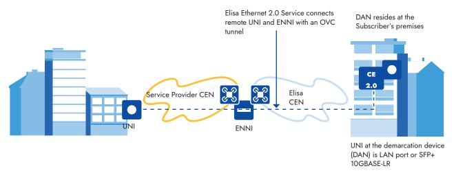
From the Service Provider's point of view the Ethernet 2.0 Service is a L2 tunneling service based on the MEF's specifications where an OVC is used to connect two interfaces - ENNI and UNI - using parameters and attributes defined in MEF 33.
