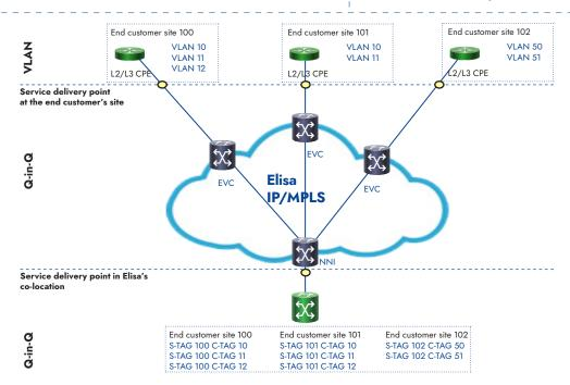
In Elisa Operator NNI Service, specific VLAN tags (S-Tag) are assigned to testing. Options for the Ethernet frame (ethertype) in Elisa Operator NNI Service are 0x88A8 (default) and 0x8100 (to be used upon separate agreement).
