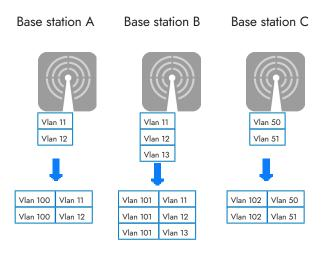
In the NNI, the frame sent by the base station is received with an additional Q header, which means that the frame has two Q headers.
